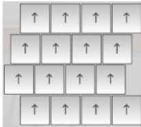
Carpet Installation Brick Ashlar
